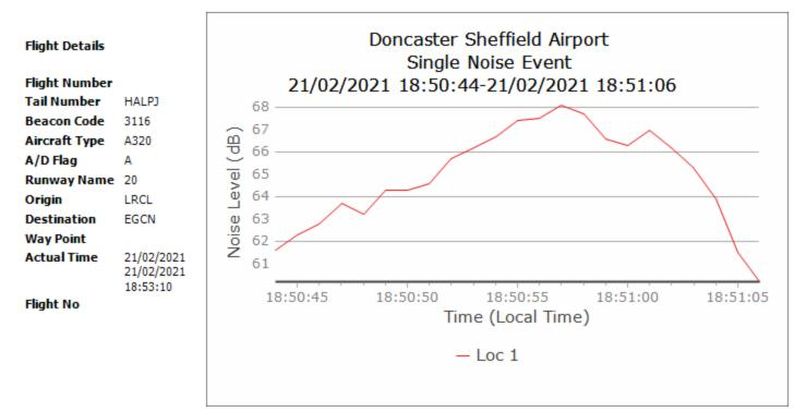
The above is an example of a Noise Event Graph from the Noise Monitoring and Track Keeping System for a Wizz Air Airbus A320 arriving on runway 20 recorded at the Boston Park Noise Monitoring Terminal.
